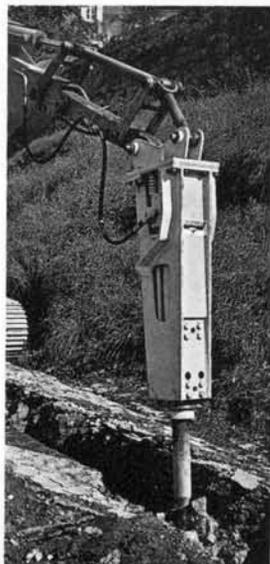
MONTABERT BRH 501 and BRH 250 Breakers have been successfully operating in Australia on excavators and backhoes for more than 18 months. These Breakers have been used for secondary breaking in quarries, rock breaking in trenches and for foundations and for demolition.
